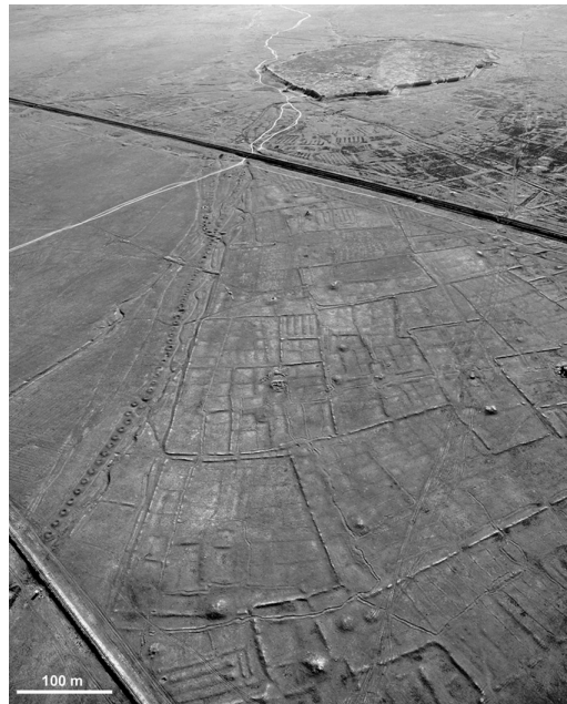
FIGURE 20.12 Aerial photo of karez line developing until the northern periphery of the medieval town of Sauran (thirteenth to eighteenth century AD). View to SE. GPS coordinates of the first well at the bottom left corner of the photo: N43°32′04.37″ E67°46′28.80″. (Courtesy of R. Sala).
